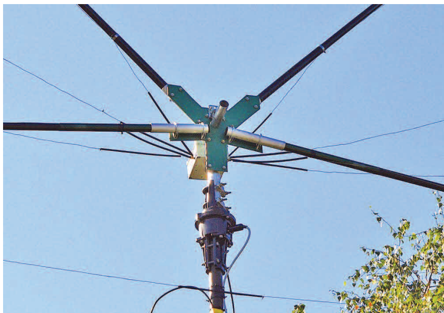
Figure 4 — Prototype antenna supported by trimmed cross bracket mounted atop a Yaesu G-450C rotator. A plastic box containing the 6:1 balun is mounted behind the cross bracket.
